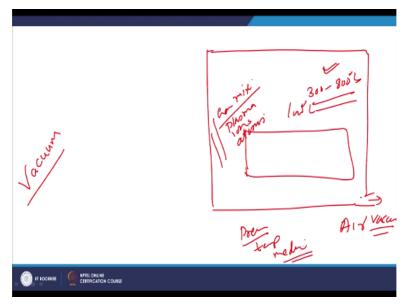
And for that there is a special category of the processes where we use vacuum. So the components whose surfaces are to be modified is kept under the low pressure conditions. So that all atmospheric gases are extracted out. So this will be used to create the vacuum and chamber. So there is a vacuum chamber which will be used to create the low pressure by extracting air and the component to be modified are placed in this chamber.
