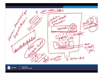
Now will be talking about the 1 particular vacuum surface modification process where vacuum assisted vapour deposition process. So in case of the vacuum assisted deposition process we use large chamber like this and this is connected to the vacuum pump to create the required vacuum and this is the chamber. In this chamber we use the heating arrangement which will be providing the required heat.
