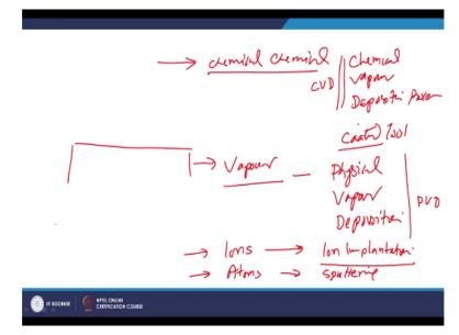
So basically there are 3 things are used for chemistry modification, 1 is the chemical reactions at the surface and this is basically used in the chemical vapour deposition process. This is used extend is this approach is extensively used in case of the like the tool inserts where multiple coatings are the single coating layers are deposited over the carbide tools. So that coated tools are basically manufactured using the CVD process.
