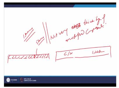
And not very thick layer of the modified composition is achieved like we have seen in case of carburizing nitriding which can be up to like 1500 micro metre for carburizing 1.5 m is very common for nitrogen 200, 300, 500, 600 micro metres also. But this is true for the carburizing or nitriding or cyaniding kind of processes but when we use vacuum based processes these are limited to very thin layer.
