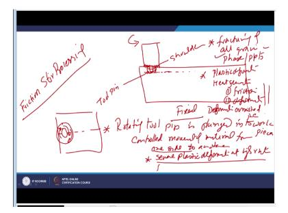
So, that method is friction stir processing, in friction stir processing like the surface whose properties are to be improved are modified using a particular tool like say this is the tool having shoulder which comes in contact with the surface and then there is a pin which is also called pro. So, this is basically tool pin and this is the shoulder tool shoulder which comes in contact of the surface.
