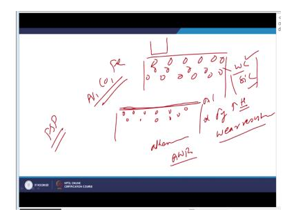
So, once the these particles are reinforce in the soft matrix then they will be able to so, provide the required support to the surface layers, will be able to provide the support to the external load whenever load is applied through the surface layers. So, basically the presence of such hard particles like tungsten carbide, silicon carbide in aluminium matrix reinforced through the FSP.
