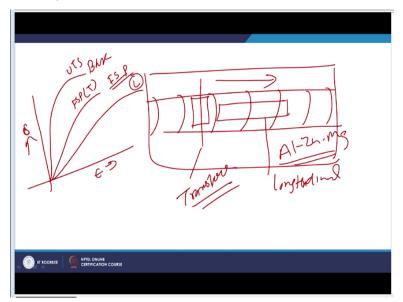
Now if we see whenever FSP is carried out there will always be like this is the surface of the substrate and FSP is carried out by passing the tool along a particular direction like this. And in this direction if we take the sample from this direction which is perpendicular to the FSP direction and if we take sample from the longitudinal direction which is the direction of the FSP. So this one will be termed as longitudinal.
