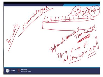
In addition to this we have also talked about the principle of the surface modification using the mechanical approach wherein the surface layers are subjected to the localised application of the forces at the surface. So, that the near surface layers are deformed plastically and this plastic deformation at the surface layers causes the work hardening, sometimes re-crystallisation of the grain growth, grain refinement, refinement of the grain.
