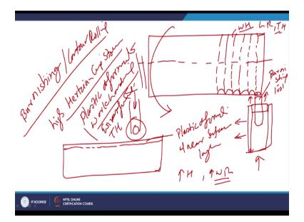
Now we will take up the another mechanical deformation or the mechanical approach of the surface modification which is like burnishing or contour rolling. Burnishing and contour rolling both processes work by and large in the similar manner like for burnishing purpose the component subjected to the like say this component is to be modified using the burnishing process.
