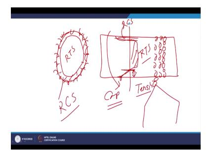
So, these 2 things which will be happening when the shot peening of the surface components is performed, let us say when a cylindrical shaft subjected to the shot peening like this with the help of suitable nozzle. So, the component which is rotating and the balls are being shot onto the component or in the substrate at regular interval, so the entire surface from all around will be subjected to the shot peening like this.
