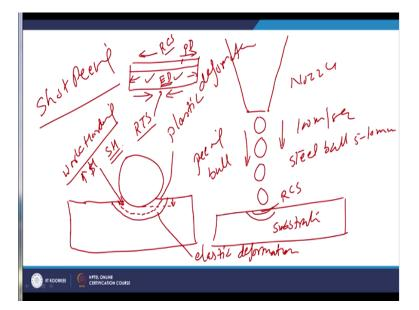
So, for shot peening basically we use nozzle through which the steel balls are accelerated at high speed like say up to 100 meter/second, the steel balls of 5 to 10mm in diameter are accelerated to the high speed and they are directed towards the surface for impingement. So, the impact of these balls with the surface causes the surface layer deformation like say this is the substrate, this is the shot peening nozzle.
