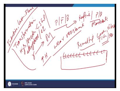
And likewise we can use a TIG hardening or the plasma hardening. But the basic principle in all these hardening processes is based on the transformation hardening wherein high or medium carbon steel or alloy steel or cast irons are subjected to the localised heating of the near surface layers. So that required transformation for austenite to the martensite can be achieved.
