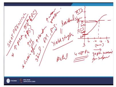
And if we try to see the depth up to which the kind of stresses as for typical example then the depth up to which the residual stress magnitude is affected residual stress. We know the residual stress magnitude can be maximum equal to the value of the yield strength of the metal. So, if the metal for metal yield strength is 400MPA then this will be the maximum magnitude of the residual stress which can be generated.
