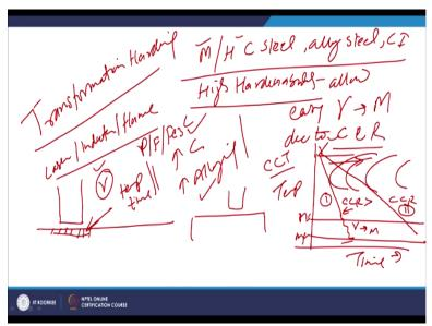
Now coming to the first category of the methods like transformation hardening, what is the basic principle in these methods. So, transformation hardening method, these method is applicable to the medium or high carbon steels, alloy steels and cast iron as I have said, these steels offer very good or high hardenability and so means these kind of the metals allow easy austenite to martensitic transformation due to low critical cooling rate.
