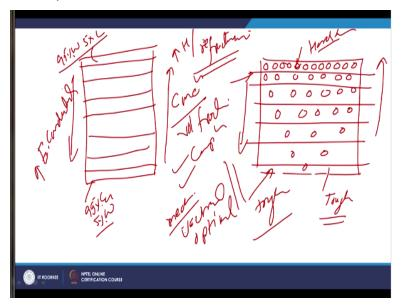
This is the one material and we are reinforcing this is the material which is soften ductile. So, this is tough material right and if we reinforce the higher fraction of the hard particle like ceramics are reinforced in very large concentration at the surface. And then concentration is gradually decreasing as we move below the surface then we will clearly notice the gradient in terms of the hardness and in terms of the toughness.
