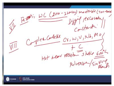
Then there is category 7 kind of the materials which are used for wear resistant applications these are also of the ferrous systems these have the tungsten carbide as a main element for enhancing the wear resistance capability the tungsten carbides offer the hardness to the tune of 2000 to the
