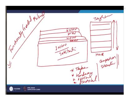
Then we need different kind of the material, say we want that material is very hard in one side and very tough on the other side. So this kind of due extremely different combination of the properties which are not available in conventional materials. So, to satisfy such kind of requirements the special category of the materials has been is being developed that is called functionally graded materials where there is a gradient in terms of the properties from one end to another.
