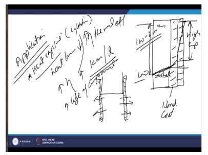
So, now schematically we will see the how the temperature variation can be observed, this is the substrate or the base material over this will be applying the bond coat like this, bond coat for good bond strength and however the bond coat the thermal barrier coating material is applied TBC. So, what we will see here that in the temperature this is the high temperature side where TBC has been applied.
