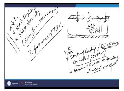
Another requirement apart from the lower value of the k and strain compliance condition where in thermal expansion co-efficient of the substrate and coating material both are largely same. Another important requirement is that the material is stable in many aspects like thermally stable thermally means at high temperature does not leads to the modification of the structure and it does not lose it is mechanical properties.
