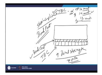
But it has been found that the thermal barrier coating materials if they have large difference in the in alpha value means if the steel is having the 12 units of thermal expansion coefficient and the material which is being used is having the like 16 units of the thermal expansion coefficient. So, this kind of the mismatch will lead to the thermal will lead to the tendency for the falling or chipping off of the coating material.
