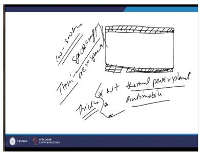
Now we know that the if the bond coat material if the TBC coating is very thin then the transfer of the heat from the outside to the substrate will be easier. So, in order to decrease the extent of heat transfer it is always favourable that the thermal barrier coating thickness is great. But since so the very thick coatings of the TBC materials can be applied in 2 situations where the weight is not a big issue.
