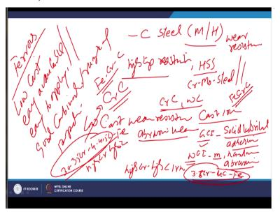
Now the most common ferrous metals which are extensively used most common metals which are used for wear resistant application is the ferrous metals. So, ferrous metals are very low in terms of the cost easily available and easy to apply. So because of these features these are extensively used and offers the good combination or the range of properties.
