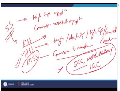
Now there are few other unique kind of the metal systems and their role is identified in a particular way. For example stainless steels, stainless steels are mostly used for high temperature applications, corrosion resistant applications. So these are the conditions then will be choosing the material accordingly again there are various categories in a stainless steel will have ferritic stainless steel, austenitic stainless steel and martensitic stainless steel.
