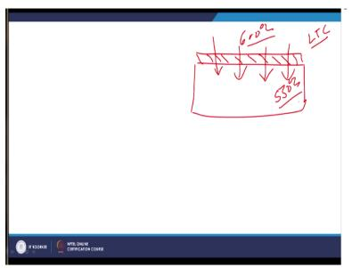
If you want that this surface will be exposed at high temperature like say 600 degree centigrade but we do not want the rise in temperature of surface above 550. So, the surface will be coated with such kind of material which will reduce the transfer of the heat from outside to the substrate. So, it will be applied with the low thermal conductivity metals and application of low thermal conductivity materials will reduce the transfer of heat from the surrounding to the substrate.
