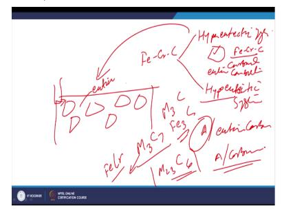
So, basically the in iron-chromium-carbon systems we have the hypoeutectic system and hypereutectic system where the big primary polyhedral shape iron-chromium-carbon-carbides are form apart from the eutectic carbides. So eutectic carbon and in case of a hypo eutectic systems basically we have the austenite and the eutectic carbides.
