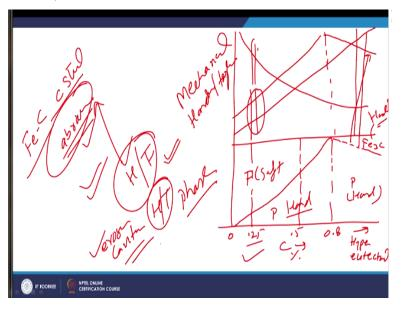
So, how does it will be leading to the variation in wear resistant we know that the chromium the carbon content in steel directly affects the phases present in the steel. And say 0% carbon, 8% carbon in the x-axis. So, there is the if we increase the carbon content there is increasing fraction of pearlite and decreasing fraction of the ferrite. So, this is the ferrite % and this is the pearlite %.
