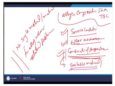
Now as far as the choice of the materials like the alloys or composites or the functionally graded materials or the TBC's which one is to be chosen for from that will depend upon the kind of the service conditions which will be experienced by a component during the service or these service will be determining the wear mechanisms responsible for material loss, in light of these things will try to see what combination of properties we should have in material surface.
