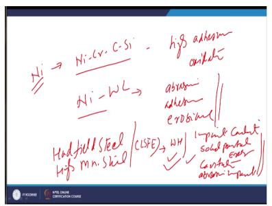
We have the nickel-chromium-carbon-silicon, this is 1 system which is normally used for good high adhesive wear resistance and high temperature oxidation resistance, nickel-tungsten carbide kind of systems are used for group at abrasive and adhesive wear resistance as well as these also work very effectively under the erosive wear conditions like solid particle erosion conditions.
