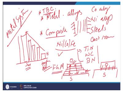
So, here if we go there are the options are the metal systems which are available, metal systems wear resistance metal systems. So, 1 is like simple metals which are basically alloys, these maybe in form of like cobalt alloy or Nickel alloy or various types of the steels cast irons etc., all
