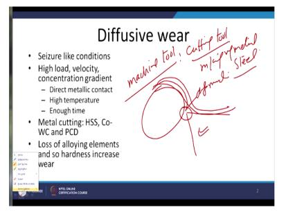
Now we will see there is a typical engineering component which is called machine tool where in machine tool the cutting tools used for machining of metals like steel, cast iron etc., so this is a tool during the machining applies the force onto the work piece. So, by sheering extend material is removed and so because of the application of the forces the deformation is involved in the cutting zone, chips are formed.
