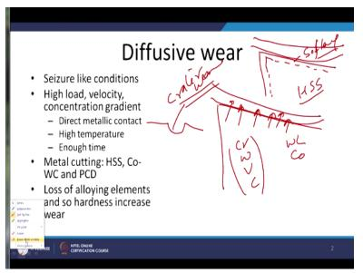
This leads to the situation where the loss of the alloying elements from the phase of the tool to the chips starts. So, the tool is having the higher concentration of the alloying element in form of like tungsten carbide, cobalt or chromium, tungsten, vanadium, carbon etc. and since the temperature is high direct metal t metal contact exist and contact is continuous. So, there is continuous tendency for the loss of these alloying elements to the chip through the diffusion.
