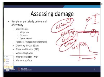
Now the hardness test is another method which shows the kind of damage which is taking place. In this case what we do since in most of the wear mechanisms like adhesion, abrasion, cavitation, erosion where some kind of the stresses will be acting at the surface. So, these stresses cause near surface layer deformation, these near surface layer deformation will be causing the work hardening.
