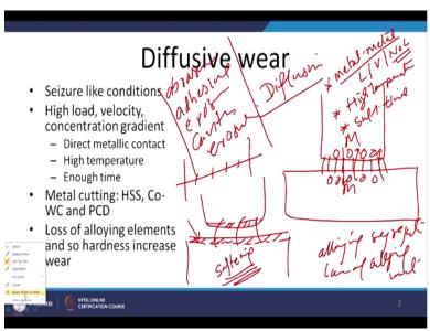
We know that in case of the diffusive wear the diffusion is the basic mechanism. So for the diffusion what is important that the components which are interacting must be in direct metal to metal contact for diffusion to take place. This is the requirement because diffusion, basically diffusion means diffusion of atoms from 1 side to another and for movement or diffusion of atoms from 1 side to another it is necessary that there is a direct metallic intimacy between the 2.
