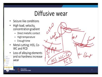
So, whenever the tool acts onto the work piece, the forces are generated, the forces will be acting near the cutting edge. At the same time the chips which are coming out of the workpiece in form of small pieces of the metals or continuous chips which are coming out they will be moving over the phase of the tool. So, due to the involvement of lot of energy in machining part of energy is converted into heat, that heat causes rise in temperature.
