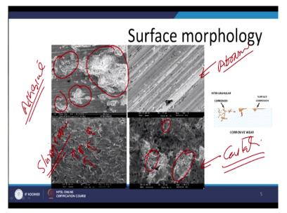
For example these are 4 scanning electron micrographs of the 4 different surfaces created by the different surface wear mechanisms like this is for the adhesive wear. Adhesive wear as I have said mild oxidative wear adhesive wear through mild oxidative wear mechanism causes the lot surface oxidation which we can see in form of these white oxides and patches, while abrasive wear will be causing the indentation and then formation of the deep scratches.
