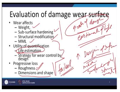
So, here this is what we say that weight, sub-surface hardening, structural modification, mechanical layer formation takes place whenever wear is taking place and this continuous progressive loss of the material during the wear causes the increased surface roughness or modified dimension in geometry of the component. And when these things happen beyond acceptable level will say that component has failed and we need the repair or a replacement of the component.
