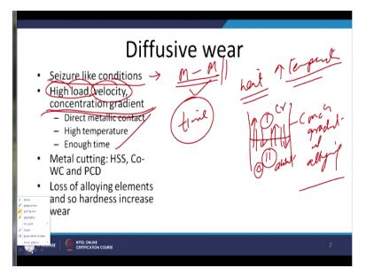
So, if we see here under the seizure like conditions, under the adhesive wear conditions means during the adhesive wear under seizure like conditions of course there is direct metal to metal contact situation. And this is facilitated by the high velocity, high load and this is the another driving force which is required high velocity and high force will generate the heat, sufficient heat and heat localisation, so the rise in temperature will be caused by these conditions.
