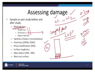
So, these are like material loss, if we have to measure the loss of the material from the component subjected to the wear or any particular kind of the damage then we can use these 3 methods for measuring the extent of the material loss taking place. So, what we will do initial weight of the component and final weight of the component will be taken and depending upon the operational wear mechanism we normally use the weighing balance accurate up to 0.1mg for the adhesive wear test.
