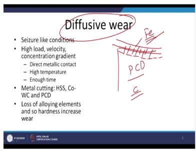
The similar kind of the damage and degradation is observed if the polycrystalline diamond is used for machining of the steel. Since in steel iron is dominating and iron is having very good affinity with the carbon, so in polycrystalline diamond which is a form of the carbon only. So, the carbon at a higher temperature starts getting diffuse out through the iron, so this leads to the again damage to the diamond tool bits in form of the loss of hardness.
