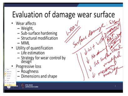
Now whenever we put any component in use we normally say that there is continuous wear and tear in the component. So, whenever a wear is taking place any component how to check the extent of damage which is taking place onto the worn out component. So, to check the surface damage on the component subjected to the wear what we should see.
