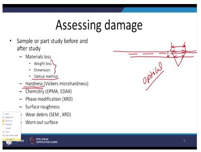
Sometimes we are not able to measure neither the dimension nor the weight if the component is very bulky, very rigid still if you want to measure the kind of surface damage which is taking place due to the surface degradation mechanisms. Then we use 1 optical method, so in that method like this is the surface, so what we will do make 1 indentation and say this is in the beginning and we will measure the this length of the indentation at the top.
