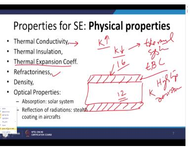
We may require so for improving the functional team, improving the tribological line we may use high conductivity metal systems as well as the low conductivity metal system. So, low conductivity metal systems are used for improving the thermal efficiency of the component of the thermal systems and thermal barrier coatings tBC these are called tBC.
