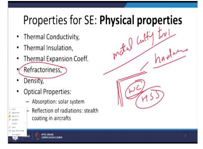
So, high temperature resistance this is important especially the coatings which are used for the in the metal cutting tools for surface modification like variety of the coatings are used over the like this is the tool can be made of tungsten carbide or made of the HSS, so the surfaces of such kind of the tools are coated with the such kind of materials which can retain their hardness at high temperature.
