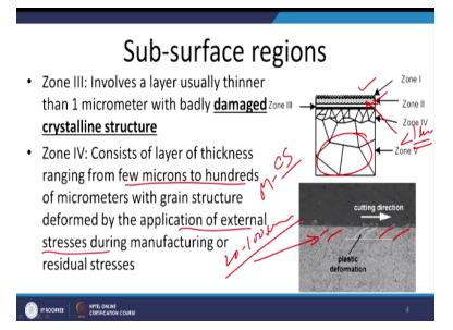
And the third zone is damaged zone we know that most of the metals will have the crystalline structure and this crystalline structure involves the regular arrangement of the atoms in one particular order and whenever metal is subjected to the mechanical processes for sizing and shaping or some other kind of the processes then like say the shot pinning or any other process used for improvement a very thin zone which is formed next to the oxidised or nitrides which are present in the second zone.
