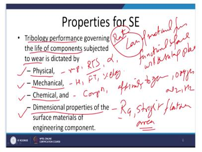
And accordingly the properties it should have that will be dictated. So but in general if we see the performance tribological performance in terms of the wear resistance of a mechanical component is influenced by these following 4 groups of the properties. So, the tribological performance which is affecting or determining the life of the component under the wear condition is dictated by these 4 group of the properties.
