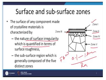
Because although there is an optimum combination very high surface roughness or very low surface roughness both result in higher friction. While the optimum level of the surface roughness results in the good combination of the wear and friction resistance. So, in general since it is very difficult to achieve very high degree of the surface finish therefore efforts are always made to reduce the surface roughness.
