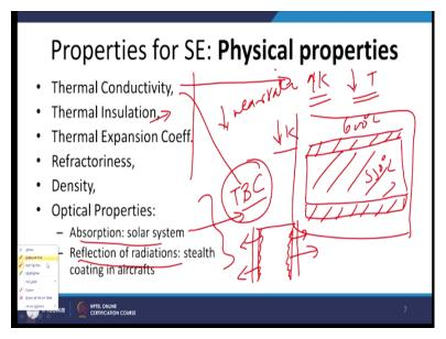
So, first of all will be looking into the physical properties and the way by which is the physical properties can affect what are those physical properties and the way by which they can affect the surface performance. They are 2 types of the physical properties 1 is which are primarily used which are primarily designed in a particular component in such a way that it reduces the wear rate.
