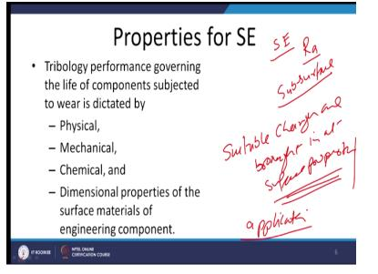
Now so as you have seen that the each surface will be composed of the 2 aspects, 1 is like the features which are present at the surface in terms of the surface roughness Ra or in terms of the kind of a the sub surface zones which are present below the surface. So, we need to for improving the performance of the mechanical component it is required that the suitable changes are brought in the metals, brought in the properties of the surface suitable changes are brought in the surface properties.
