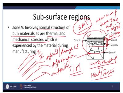
So, the zone 5 involves the normal structure of the bulk material as per the thermal and mechanical history or the stresses experienced by the metal during the manufacturing. So, this is how we can say there are 5 zones those the zone 1 is of a absorbed gas or the hydrocarbons or
