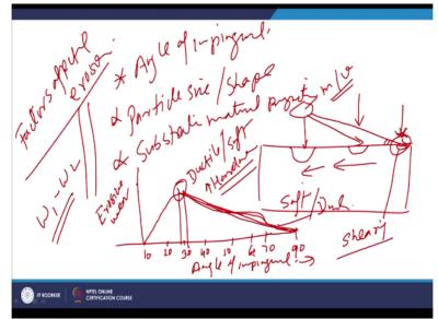
So angle of impingement and the workpiece material properties these are the 2 crucial parameters which govern the loss of material from the function of surfaces by erosion another important aspect here is the factors which govern the erosive wear so factors affecting the erosion. So factors affecting the erosion includes like angle of impingement of the particles.
