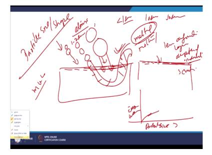
So this is 1 aspect and the second aspect is about the particle size. So particle size and shape, now the erosion can be placed through a very wide range of the particles it may be in form of the atomic size of like say less than 1 micrometre or 10 micrometre or 50 micrometre, so they are very large size range. So whenever the atoms are directed on to the surface like in electron beam or ions when they are directed on to the surface will be seen that the surface layers.
