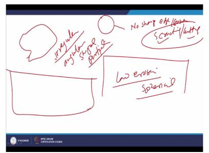
The shape of the particle is the another aspect like if the surface of the workpiece is subjected to the impingement by the spherical particles since it has a no sharp edges corners to cause a
