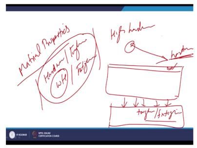
So as far as the material properties are concerned it is not just good to have very high hardness, it is required that the material should have the good combination of the hardness, toughness, work hardening behaviour and the fatigue resistance. If material is having these characteristics then in general under the normal conditions of the reason it will offer very good erosive wear resistance, but since many of these are the contradicting properties.
