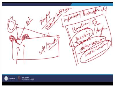
So this is 1 aspect as far as the erosion is concerned. Now as per as the different factors that affect the erosion is so in this case apart from the indentation and surface layer plastic deformation which will be governed by the hardness, yield strength of the material. The other factors that determine the material loss by the erosion is also the ductility, toughness, fatigue resistance and work hardening tendency.
