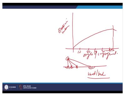
The another plot where angle or impingement in the x-axis and erosive wear on the y-axis, in this case at low angle we know that if the material is hard and brittle. So with the low angle of impingement there is not much depth of penetration not much scratching. So the wear it is less, so like say 10, 30, 50, 70, 90 degree of the angle of impeachment. So limited depth of indentations is very less.
