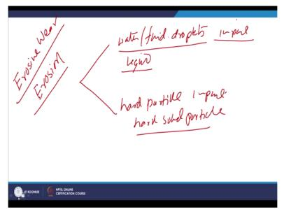
So the topic is erosive wear, the mechanism by which material loss in this mode of wear takes place is the erosion and this is caused by the 2 types of the situations 1 when the water or fluid droplets moving at high speed impact with the surface of the component being considered or hard particle impact or impingement of the hard particle on the surface of the workpiece takes place.
