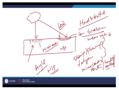
So if we see the soft and ductile materials it is the fatigue resistance the ductility which will be important and the work hardening behaviour which will be important to look into the way by which material is being removed from the functional surfaces. On the other hand if we take an example of the hard and brittle material. In case of the hard and brittle material like this.
