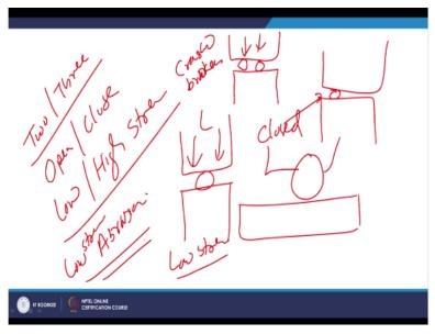
And then there can be open or closed type abrasive wear where hard particle comes between the 2 firmly placed components or surfaces like this then it leads to the closed 1 or 1 hard particle firmly held and pressed against the another component like (()) (01:48) and wherever polishing is performed. So that forms that close abrasive and when the abrasive particles are allowed to move freely then over the metallic surfaces then it leads to the open abrasion.
