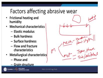
So these factors will be affecting the abrasive wear. For example if some kind of the heating is taking place of high temperature will be lowering the hardness of the surface layers reduction in hardness will be increasing the abrasion tendency and so the abrasive wear will be increasing. Similarly the material related factors there are 2 broad categories as per is the metal is concerned mechanical properties and metallurgical properties of the material.
