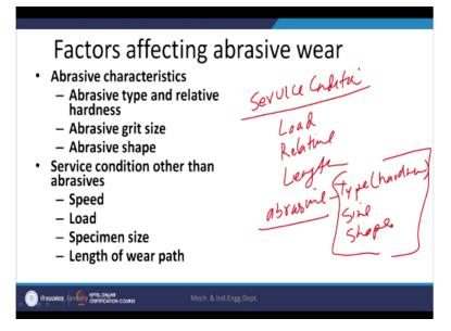
Service condition related factors means what is the kind of the load, what is the kind of the relative speed of the abrasive particles, what is the distance travelled are the length which will be covered by the abrasive during the surface, then what are the kind of the abrasives which will be interacting with the surface of the material like their type of abrasive affecting or determining their hardness.
