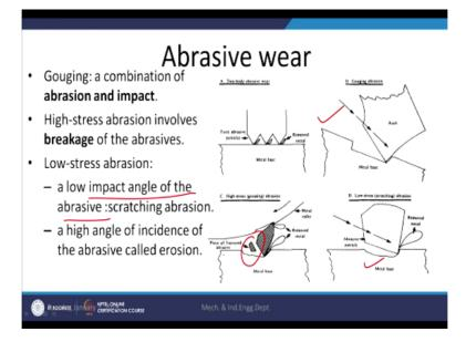
High-stress abrasion wear particles get crushed and lowest stress abrasion particles largely retain their size and shape but remove the material by abrasion through the metal cutting or the ploughing. So in case of the lowest abrasive the low impact angle causes the scratching abrasive while the high angle of the incidence causes the erosion.
