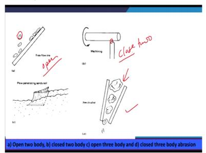
So in which way we can express and how is schematically we can understand these wear mechanism for that we need to see certain diagrams. So again going back to that what we have talked this is the open abrasion system this is a open abrasion system where open two body abrasion, if the abrasive particles falling freely on to the surface. So this is open two body operation system.
