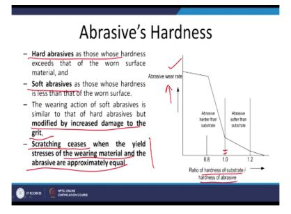
So if we ou compare the hardness of the abrasive and work material that we can find the ratio. So ratio of hardness of the substrate and hardness of the abrasive. So if the hardness of the substrate is less and hardness of abrasive is more then it will be causing the higher wear rate. So greater is the lesser is the value of this ratio greater with abrasive wear rate or abrasion of the material. If the 2 are very close the substrate hardness and the abrasive hardness is very close.
