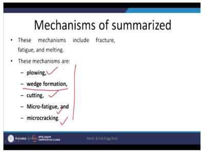
These are the 5 different mechanisms about which I have set the ploughing, metal cutting, micro-fatigue, microcraking which formation also sometimes takes place but these are the two mechanisms which do not contribute much towards the material removal by enlarge the material is displaced plastically. So in this case is this one plowing mechanism where like over a soft metal we forcefully penetrate 1 tool.
