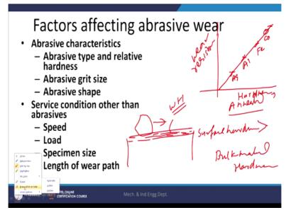
The second phase particles like matrix is a soft and tough while ceramics particles are other particles second phase particles which are hard and brittle. So in that case a combination of the ploughing and the microcracking will be observed. These are some of the characteristics all the factors which will be affecting the abrasive wear of the material. So now we need to see one simple diagram how the material hardness changes.
