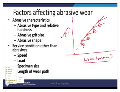
So it will be going like this for the pure metal hardness variations say for silver, aluminium, iron, cobalt. So when we work hard in the material this is for the pure, when we work hard in there is increase in the hardness. So hardness will be increasing as with the deformation. So what it is showing there is a division from the hardness of the material in the anneal condition hardness increases.
