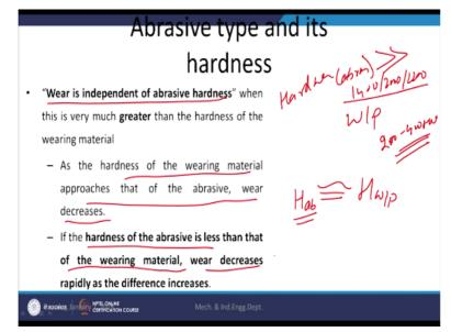
So when the hardness of the abrasive is too high, hardness of the average is significantly higher than the work piece like abrasives which are harder than maybe like say 1400 hvr 2200 or 2200 hv so it is very hard abrasive as compared to the workpiece which may be like 200 to 400 HV hardness values. So here if the hardness of the abrasive is very high then it does not affect the abrasive wear behaviour appreciably.
