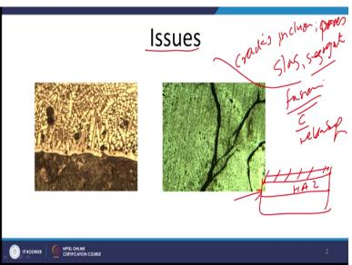
There can be inclusions, there can be pores or porosity, there can be slag inclusions or so, these are some of the issues. There can be segregation of some of the elements these are the issue which are associated with those surface modification techniques where fusion is involved. And sometimes if the lot of heat is applied during the surface modification like in processing like carburizing or weld surfacing.
