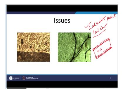
So, for this purpose we will making the major component of the low quality material like mild steel. And then surfaces will be modified using those techniques those material which can help us to have all those functionalities required for good performance of the product. So, in that case instead of making the entire component of the good quality material only the functional surfaces are modified.
