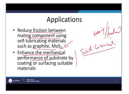
The surface modification is also used to reduce the friction between the mating components and for this purpose whatever the bearing or the functional materials are there. They are reinforced with the graphite and the molybdenum sulphide. So, the bearing materials and all the components which are used for making such kind of the mating components, these are reinforced with the graphite and the molybdenum sulphide.
