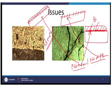
So, we have it is intended that not much of the melting of the substrate will be taking place. But the coating will have the coating may have the completely different composition than the substrate material. In that case sometime one a segregation of the alloying elements near the interface takes place. And this can be a problem under the certain conditions this may be too hard or this may be too soft zone formation.
