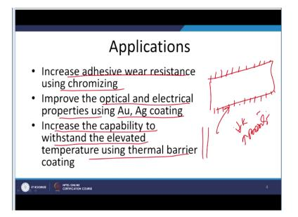
To increase the adhesive wear resistance like in normally in automatic components the chromizing is used and to improve the optical and electrical properties normally the coatings of the silver and gold is used. And for improving the optical properties suitable kind of the materials are also used for development of the cladding to increase the capability to withstand at elevated temperature thermal barrier coatings are used.
