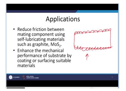
Under this category basically, I will take over a simple example like the mild steel having the say somewhat lower strength. So, if the high strength material is coated at the surface. So, this will increase the load carrying capacity it will delay the nucleation and growth of the crack at the surface. So, such kind of the methods are used for enhancing the mechanical properties and the performance of the component.
