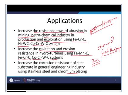
Now as for as the application of the surface modification techniques is concerned it is used in very large scale for variety of the purposes. Here we have certain examples where the surface modification techniques are used for improvement of the tribological life of the component like increasing the resistance towards the abrasion in mining, petro-chemical industry in petro-chemical industries especially in production and exploration.
