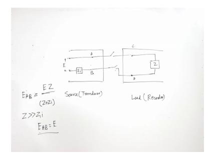
E A B because here also there is a resistance, here also there is a resistance. So, E A B is going to be total E right, divided by total resistance this will give the current right.
