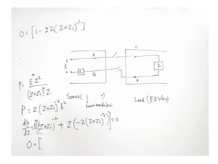
Now, they will also change source will be a power amplifier, power amplifier and recorder, a recorder maybe a electro dynamic vibrator, electro dynamic vibrator right. So, the instruments have also changed. So, this is the maximum power which is either the power which is transmitted to the load.
