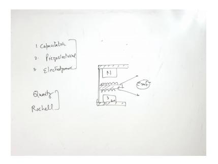
So, when pack pressure is exerted on the core, there is a movement in the core. When there is a movement in the core it is in the magnetic field there is a movement in the core EMF will be generated; and these type of I mean microphones are found I mean the microphones with this electro dynamic arrangement are found in many of the applications or many of the devices in day-to-day life.
