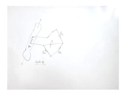
So, the principle of a strain gauge is the change in the resistance with the application of a stress, when the when the wire is pulled, when a wire is pulled its cross section area reduces and the length increases. Both the cases, lead to the increase in the resistance of wire, right.
