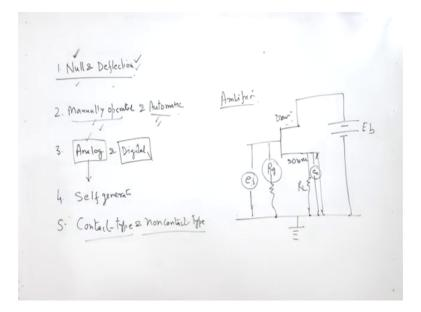
There is an electronic amplifier the function of amplifier is to increase the output right so there is a field effect transistor. So, here drain this is source and there is a input voltage this is resistance, then this is a battery the battery is and here we get output and this is r l.
