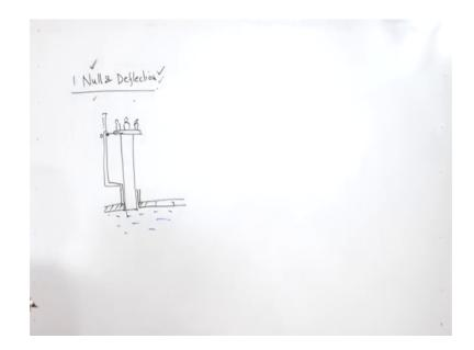
And in the vessel a pressure gauge dead weight type of pressure gauge is fixed, there is a shaft this shaft is in contact with fluid which is occupying this vessel. And the shaft has a platform and on platform we put some dead weights right, and these dead weights are and this platform is connected with a indicator.
