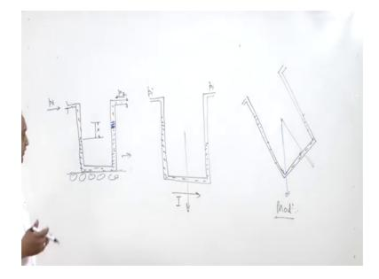
Let us take case of a manometer. So, in a manometer there is a tube right, and normally they are there is a base fluid and this is p 1 and this is p i initial pressure.
