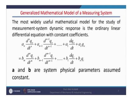
We will start with a generalized mathematical model of measuring system and generalized mathematical model starts with.
