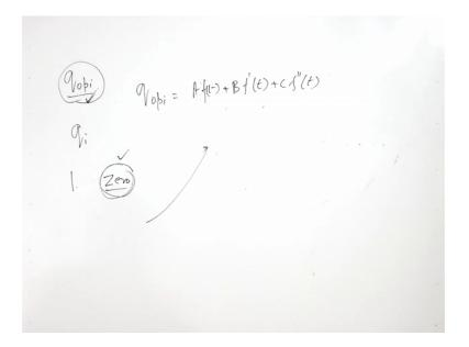
And q o p i, there is no universal method to find q o p i; the reason being need that this particular integral will depend upon the nature of input signal. It will entirely depend upon the nature of input signal. So, there is no universal method to find the particular integral that is first thing.
