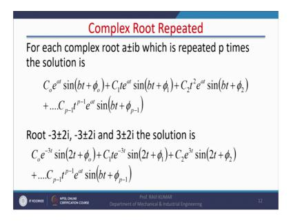
When the roots are complex and repeated, in this case the solution is going to be C o e raise to power at sin b t plus phi o plus C 1 t e raise to power a t sin b t plus phi 1 and so on.
