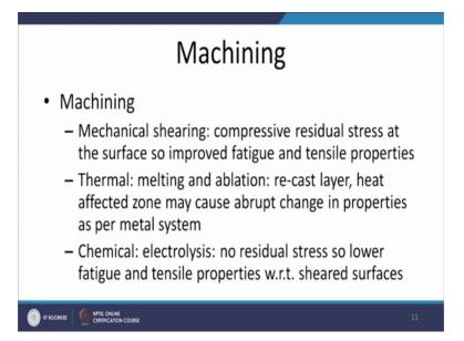
Now, the another process is the machining one wherein we know that machining can be carried out by various approaches and these approaches they are three category of the process for removing the material, one is mechanical one.
