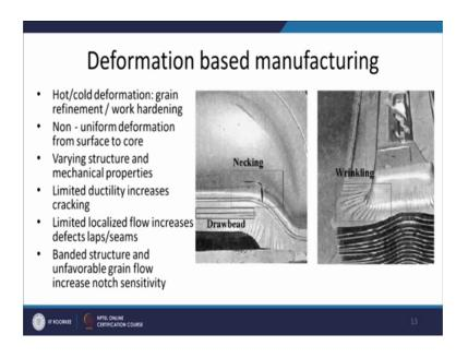
Now, coming to the deformation based manufacturing processes, we have the two broad categories; in that deformation based manufacturing process one is a hot and another is cold deformation. We know that the two processes work on the different principles, strength in case of the hot deformation based processes is obtained, so, the grain
