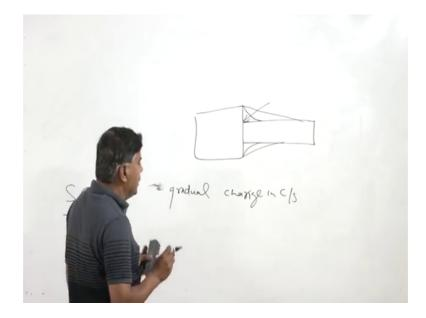
So, a stress concentration effect can be reduced through the use of through the gradual change in cross section we need to adopt all those methodologies which will help to have the gradual change in cross section like say a change in from large diameter to the smaller diameter in which way the change is been acting accumulated, either, we are giving the gradual tipper like this or we are giving a continuous curve or some fillet is given.
