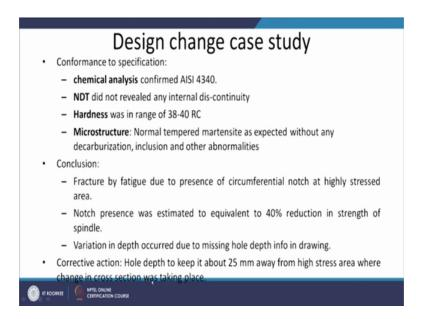
So, in order these this is about the macro examination the macro examination suggesting the beach marks and the fracture due to the overload and the beach marks or clam shell marks initiated from the root of the hole where there were feed marks conformance to the specification means we need to confirm really the material of the spindle was same as recommended or not whether properties, it had our acceptable or not whether the microstructure was proper or not.
