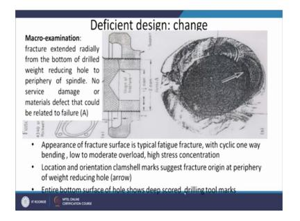
So, if we see the macro examination of the field component showed that fracture extended radially from the bottom of the drilled weight holed from the bottom of the hole a drilled for weight reducing to the periphery of the spindle.
