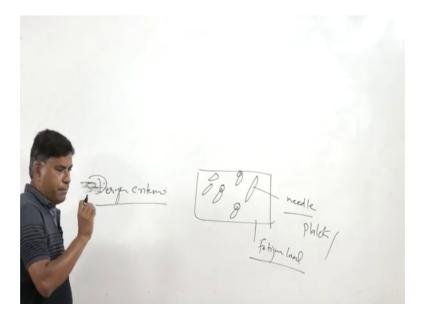
Say like say sometimes despite of everything being fine if the material metrological properties are unfavorable like the component, a is made of the material having large number of high aspect ratio micro constituents in form of a, like say in needles or the platelets or the then these will cause the higher stress concentration at the tip of the micro constraint in the matrix interface and which will easily nucleate the cracks especially under the fatigue load conditions.
