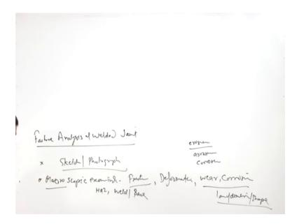
So, we can use the sketches for this purpose, we can take the photographs to support the evidence regarding the location where from the failure has taken place where the weld joint was located. Then macro examination is the next aspect, macro examination basically in helps us to see the, what was the broader mechanism by which the failure of the weld joint has taken place.
