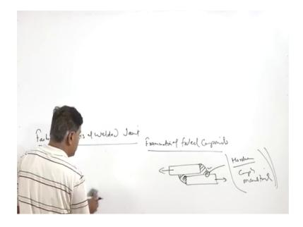
Apart from this one if the failure is occurring not exactly from the base metal or from the heat affected zone, but if it is occurring from the next through the weld metal or from a particular location like toe of the weld.
