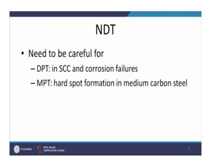
But in the 2 cases especially the DPT which indicates the surface discontinuities and if the failed component or the weld joint failure has taken place due to the stress corrosion cracking, wherein there is a possibility of the presence of the corrosive media in the in the fracture surfaces then DPT is to be avoided because, the liquid of the DPT test can get filled in and then it can create confusion with the corrosion media.
