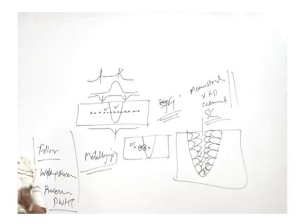
So, this is what can be identified to some extent through the metallography of the of the weld joint. So, like say this is the weld joint and if we do the metallography we can have the microstructure of the base, heat affected zone of the fusion boundary and also of the weld centre. So, these will help us to indicate whether the penetration has been proper or not at the fusion boundary or whether the kind of the phases which are being formed at
