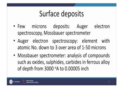
Then for analyzing the surface deposits there are two techniques. So, Augar electron microscope is used for determining the for measuring the elements up to the atomic number 3 over the area of 1 to 50 micrometer, while the mossbauer spectrometer is used for analysis of the compounds are like sulfides carbides and oxides present in the ferrous systems and which can analyze the depth up to three from depth of varying from 3000 angstrom to the 0.00005 inch.
