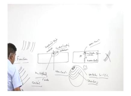
Similarly, now the there is one more fracture; which about which we need to talk is the fatigue fracture. This is related with the basically the determination of the fracture only. So, here we know that even the fatigue can occur not just on the components with the stress regions like this, but also the components which are very smooth.
