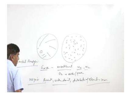
Embrittlement of the like presence of the hydrogen, nitrogen in iron leads to the especially high strength steels it leads to the embrittlement.
