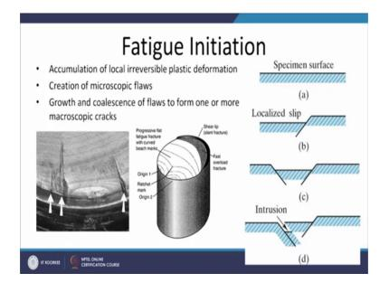
So, that will be leading to the creation of the intrusive and extrusion and these intrusions and extractions will be acting as a stress raiser and thereafter once the sub crack a stress raiser or the crack like defect has been formed of sufficient size, then the growth of the crack will be occurring in a particular way.
