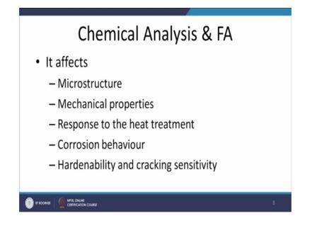
And not just that the corrosion resistance of the material is also affected because if the homo composition is homogeneous, then corrosion resistance will be good if there is segregation of some of the alloying elements either the grain boundary or within the grain, then it will be it will be forming the galvanic cells easily and which in turn will be reducing the corrosion resistance.
