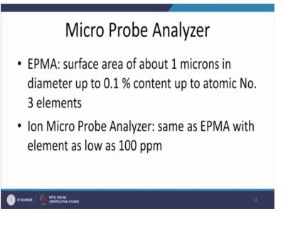
Then there are two good approaches which are used for determining the distribution of the elements in the metal like EPMA which is called electron probe micro analyzer or ion micro analyzer this is. So, EPMA is used for elemental analysis over of the surface of the diameter of one micron for analyzing the components analyzing the elements down up to the three atomic number and the content is up to 0.1 percent.
