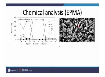
Now, we will see this is the line analysis where that the between two points one line is drawn and the analysis is carried out between these two points and the distance between the points which are to be analyzed can be selected suitably.
