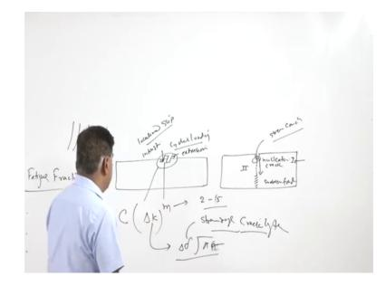
So, the da by dn is the typical formula, which is used to indicate C is the constant and delta K is the stress intensity factor range m; m is the constant.
