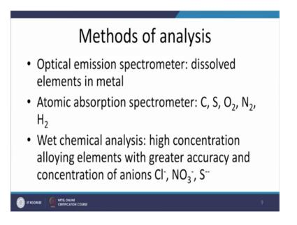
Now, there are various methods, which are used for the chemical analysis purpose depending upon the purpose what is to be analyzed in what size what quantity which material is there to be analyzed, we have the different things like optical emission spectrome metry is used for determining the elements dissolved in the metal.
