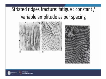
So, as I was talking about that the striations are formed and which spacing between, which indicates that roughly the value by which the crack will be growing in each load cycle and the it can be constant or variable the constant stress amplitude results in the constant spacing otherwise it can be fluctuating for given uniform for the given material properties.
