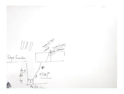
So, this indicates the rate of the crack growth especially in the second stage.
