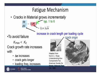
So, this is what I have just explained that the crack growth rate, can be expressed using such kind of the equation which is known as a power law, and crack growth rate of course, increases with the increase of this stress range, which is clear from this diagram because delta stress range in as the stress range increases the stress intensity factor range also increases, which in turn increases the crack growth rate.
