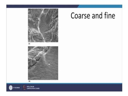
And if there is a heterogeneity in metal properties of course, the spacing can also vary according to the kind of material through which crack is passing; the course these striations can be coarse or fine striations will indicate that the crack is growing at a lower rate, while the courses is striations means the coarser or wider spacing between the striations, indicate that the crack is growing at a faster rate
