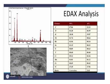
This is the EDAX analysis which is carried out with the help of fesem and here this area is analyzed to see what is present in what quantity. So, this is the kind of analysis of the different elements of this particular area.
