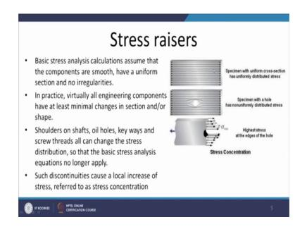
Stresses are uniform and this stress flow lines are equally distributed, but whenever there is a like say in this particular case, when there is a hole and around the whole the stresses are more steps for lines are more localized there more crowded indicating that stress is more localizing. And this kind of a stress distribution can be seen in the third diagram where, more stress magnitude is higher near the edges of the whole as compared to the distance away from the stress raisers.
