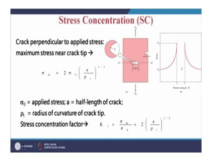
The same thing we can see now, as there is additional aspect like the geometry of the a stress raiser. So, in this case, if we see, like say, this is a simple plate of a particular dimensions like say, there is a width v and maybe thickness t that will be there. So, which all though it has not being explained here, but like in this plate is having the stress raisers of the 2 types one is stress raiser is inside and another stress raiser is at the is present at the surface.
