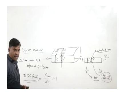
Due to the stress raiser and the reference stress that is the sigma r this ratio is termed as theoretical a stress concentration factor. Normally, when there is no stress raiser, this ratio maximum stress and reference both are equal. So, it is 1, but whenever there is a stress raiser, the maximum stress is will be high or greater than the references stresses and then stress concentration factor will value will be obviously, more than 1.
