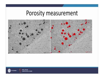
Image analysis of one particular weld joint here what it shows a darkest parts are indicating the porosity and image analysis and when image analysis carried out all these darkest parts are selected and their fraction can be identified.
