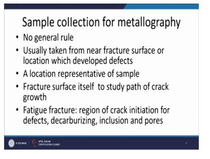
So, for the metallography we need 1 sample and sample need to be collected from the failed component, as far as the collection of the sample is concerned there is no fixed
