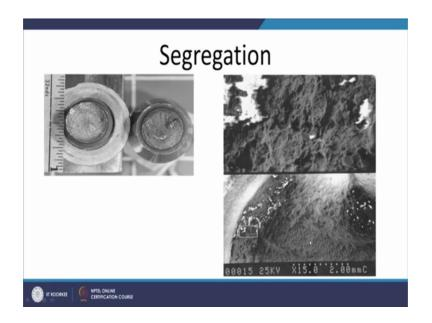
So, such kind of the variations lead to the lot of heterogeneity and variation and mechanical properties in which under unfavorable conditions of the loading easily facilitate the nucleation and the growth of crack here is another example of the segregation way which is leading to the presence of the undesirable constituents at a particular location, which are facilitating the nucleation and then nucleation of the crack and then the fracture.
