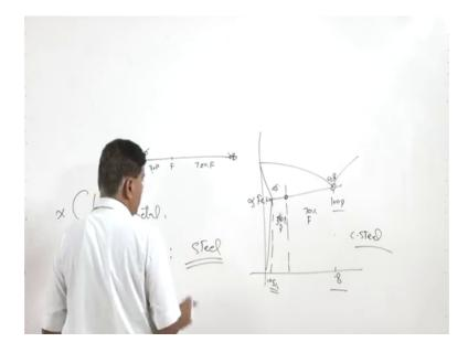
So, will take up a one typical example to understand this like in case of the steels we have the phase diagram of this kind, where this is corresponding to say eutectoid point where we have the 100 percent pearlite and this is corresponding to the 0.05 percent of the carbon, where we assume that the ferrite this side we have alpha iron or the ferrite and between these two.
