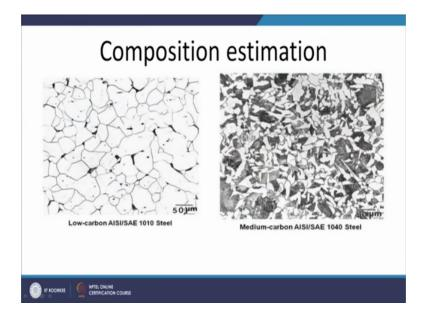
So, this dark phases at the boundary of the light etched ferrite is indicating the pearlite and the fraction of pearlite is very less and this is corresponding to the 1010 is steel, which is indicating that it is having very low carbon that is 0.1 percent carbon say it is a plane carbon steel and another one is 101 1040 is steel which is indicating where there is a 0.4 percent carbon.
