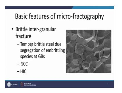
And this kind of the fracture is observed like say in case of the temper brittle steels, due to the segregation of the embrittling species at the grain boundaries this kind of fracture is also observed in case of the stress corrosion cracking and hydrogen induced cracking.
