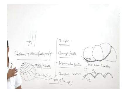
Inter granular fracture is the typical one where the crack if it is present that will be propagating through the grain boundaries.
