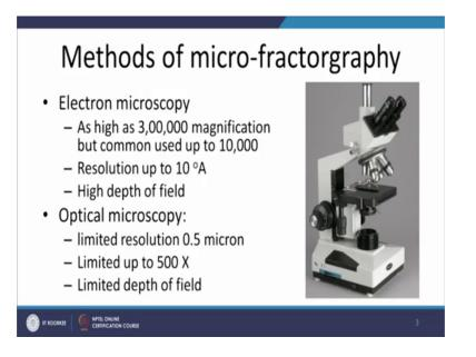
So, although we have the microscopes of the higher range also we are like 100 400 to the 1600 magnification.
