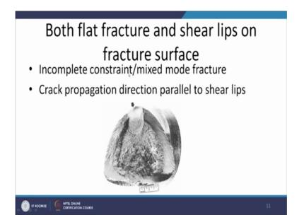
The case where the both flat fracture and the shear lips are present on the fracture surface this is called a mixed mode fracture and this is the situation where the strain is incomplete the actually plane strain conditions exist at the center. Here in this case and the plane stress conditions will be existing at the near the surface.
