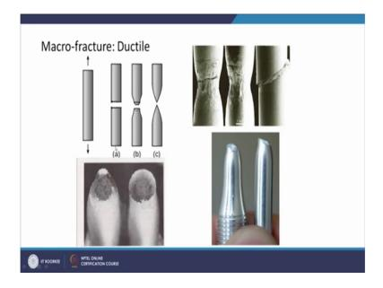
So, the a is the case of the brittle fracture, where the fracture surface is perpendicular to the axis of the loading. This is the case of the somewhat ductile fracture means partially ductile fracture in this case a at the center the we have the at the center we have the brittle fracture; that there is the flat fracture and at the sites we have the slant fracture.
