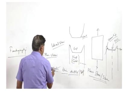
Like a tensile sample like this when subjected to the external loading and the failure occurs, when failure occurs what we find that fracture surface is of these kind of feature wherein at the center of the specimen the there is a flat fracture surface and at the sites near the surface there is a slant or fracture surface or shear lips are present.
