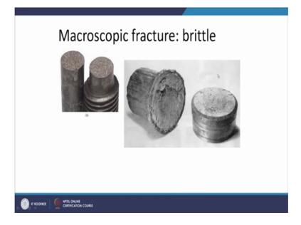
In case of the brittle fractures as I have said there is no change in cross section of the component. And so, here you can see whatever is the cross-sectional area here the same is here there is no reduction in diameter. At the same time ah, the fracture surface is also perpendicular to the externally applied load and. So, these are the 2 important features apart from the color texture and the roughness that about that we will be talking later.
