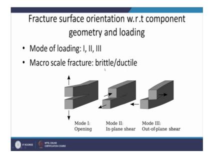
Now another information which can be gathered from the surface orientation of the fracture surface orientation with respect to the geometry of the component and the loading. So, here what we can see the fracture surface orientation like this is the component so the fracture surface may get filled like this so here this is the case of the loading one or the loading of mod 1.
