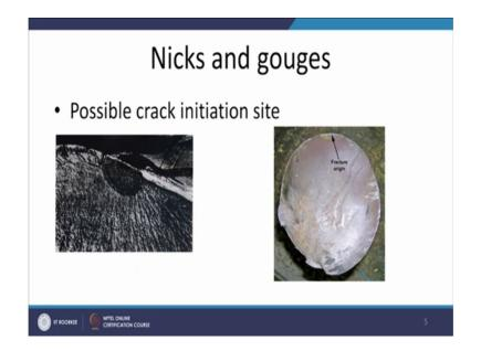
Now, as I said among the various other things or various points about which information can be gathered from the microscopy of the fracture surface, the one is about the fracture initiation site.
