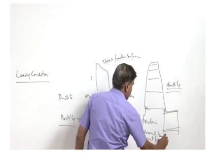
So, the square or you can say the fracture surface is normal to the external loading. then third one is like the macroscopic observation with regard to the mode of the fractures say for based on the micro scale or microscopic observation the ductile fractures. (Refer Slide Time: 31:14)
