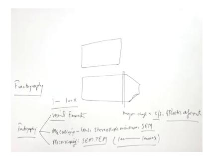
And when these observations are carried on it reveals lot of information; like if the failed component is really very big and if it has a failed like this and end is showing, in this manner what it will be showing that cross section actually of the component has reduced significantly.
