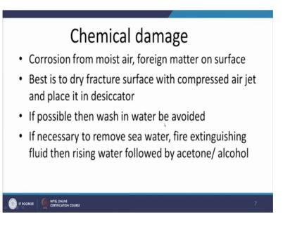
So to avoid that we need to do the cleaning under the water and thereafter like cleaning using the acetone and alcohol and thereafter after drying it can be kept in the dry place like desiccators; so, that no further damage of the surface takes place.
