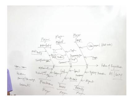
Which will have a given desirable or undesirable effect say it is coming out after the design analysis stress razor is one of the possible thing then hardness from the material side and the manufacturing side say it is coming out to be the pouring temperature which can really have the possibility of the cold shaft due to the complexity of design or it can be the like shrinkage cavity shrinkage cavity in the casting which can also lead to the failure of the component.
