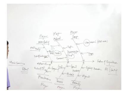
Or indicated through the lines like this as per the number of causes various lines will be plotted and all these will be connecting to the horizontal line which is showing all these are basically causes and then right side we have effect say the aluminium engine block made by casting process.
