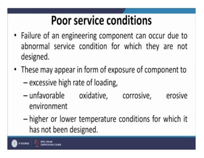
Now, the next is that poor service conditions we know that whenever a component is designed that is designed for a particular set of the service conditions.
