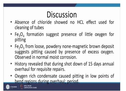
So, after this analysis it was observed that absence of the chloride showed that no HCL effect used to used for cleaning of the tubes because the HCL was being used for cleaning of the tubes and remove the dust and the rust Fe3O4 formations suggest represents of the oxygen is limited for the pitting and Fe2O3 formed the loose, powdery none-magnetic brown deposit suggest the pitting caused by the presence of the excess oxygen and which was observed in normal moist corrosion pits which were there.
