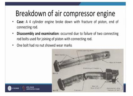
The breakdown of the air compressor engine which was full which was made from the four cylinder engine this engine actually broke down with the fracture of the piston on the connecting rod and side and the disassembly when the system was opened it was found system was opened for examination it was found that that the failure occurred of the two connecting rod bolts used for the joining of the piston and connecting rods.
