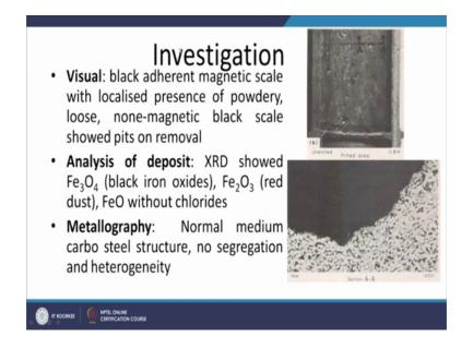
So, they wanted to investigate what lead to the failure of the premature failure of the super heater tubes. So, the tubes over cut and it was found through the visual inspection that black at adherent magnetic scale with the localised presence of powdery loose. So, both type of the black and both types of the oxides were found black adherent magnetic scale with the localised presence of the powdery loose and non-magnetic black scale.
