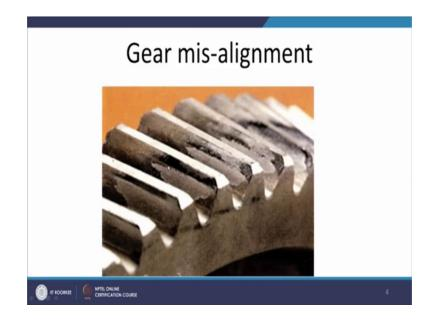
And in this particular case what we can see here mis-alignment will be leading to the increased contact in one side and another and the noncontact in another side of the gear.
