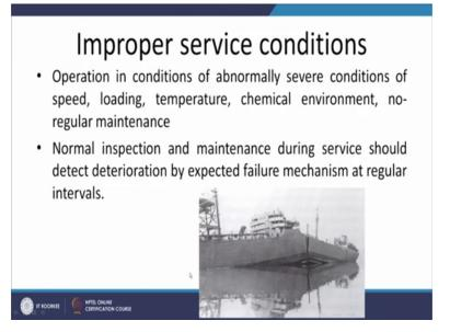
Similarly, the high and low temperature conditions for which it has not been designed can also lead to the failure of the component. This one typical example where one ship which was made of the medium carbon steel which did not have much low temperature toughness when it heat the iceberg under the low temperature conditions.
