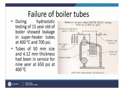
So, actually the boiler for the details if you go the boiler tube failure the failure of the boiler tube here. So, these are the super heater tubes and these started leaking during the trail run, and the trial run was conducted after the maintenance during the hydrostatic testing of 15 year old boiler showed the leakage in the super heater tubes and the tubes were operating at 400 degree centigrade and 700 psi.
