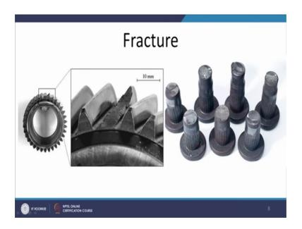
You can say these are the gear shift the gear is subjected to the overloading and the fracture of the teeth can take place, this kind of fracture of course, in normally it is a fatigue in nature where crack will first nucleate and then it will grow gradually during the service and ultimately to lead into the suppression or catastrophic of failure of the gear teeth's; so, now this is the kind of wear where loss of dimensions take place.
