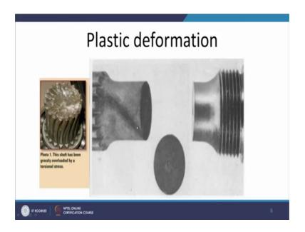
We can see here also like this by spiral feature indicates that other component as deformed plastically under the torque conditions or the twisting load conditions, then another failure is where the creep takes place the creep is a phenomena like this is.
