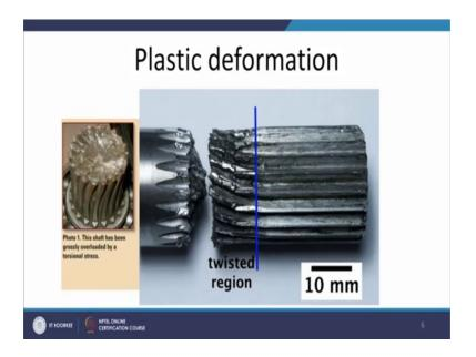
Ah then it will be leading to the malfunctioning of the walls and that will adversely affect the functioning of the automobile or engine or another is a plastic deformation where due to the excessive loading when the stresses go beyond acceptable beyond the yield strength level, then it will lead to the this what we can see here it will lead to the deformation.
