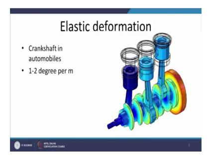
Now, we will see this is the typical case of the elastic deformation where during the operation the torque is transmitted from the engine to the through the crankshaft to the eventually to the wheels of the automobile and here the due to the transmission of the torque elastic deformation of the shaft will be taking place and if this elastic deformation is beyond the acceptable limit.
