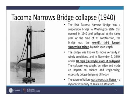
And then there is another accident which happened again in USA around 1940. This is called Tacoma narrow bridge collapse, all this was the third world's third longest suspension bridge in terms of the span length and that bridge used to flutter under the influence of the air. So, under the conditions on the of the wind velocity of 40 mile per hour this was fluttering to such an extent that it collapsed and this collapse was caught in
