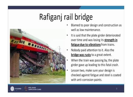
Then there is one example of the Rafiganj role rail bridge here also it was the failure was blamed to the poor design and construction and the low maintenance conditions and it is said that the plate girder decorated over a period of time.
