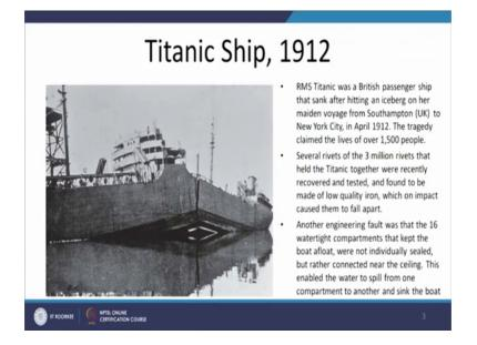
This af failure of the ship a lead to the a loss of the life of more than 1500 people and this failure primarily occurred due to the failure of the rivets this had more than 300 million
