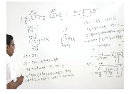
So, this is inertia J 1, this is J 2, this is damper with damping coefficient D 1, this is D 2 and here is applied a torque to the first inertia T that is function of time and the degree of freedom theta 1 t and here is theta 2 t, this spring has stiffness K.
