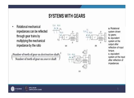
So, we have one damper which is spring and inertia. And here is input shaft, there is a gear that contain N 1 number of teeth. And input torque T 1 is applied here and there is the input angular displacement theta 1. Then here is gear 2 that is on the second shaft, there is Inertia, Damping and Stiffness.
