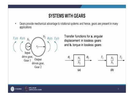
Now, we come to the another mechanical systems. They are more applicable in mechanical components that are the gear trains. So, because gears provide mechanical advantage to rotational systems and so, they find frequent applications in several applications. So, we can understand how we can represent the impedance of gears, how can we find the transfer function that contains gears. So, if we have 2 gears here.
