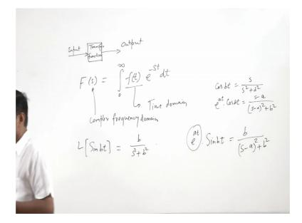
Can be represented here as; input, output and here is the transfer function. So, to find the transfer function we need to use the Laplace transform because Laplace transform is a technique that can be used to convert the differential equations or integral differential equations in time domain to algebraic equations in complex frequency domain.
