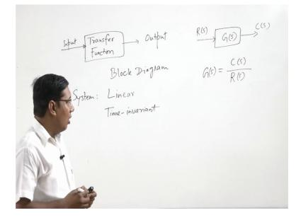
A block that takes the input so, it takes some input and it gives some output, because every system in physical any physical system that comprises with many subsystems and we give some specific input to the system and that input it passed to the subsystems. So, each subsystem has some input and then output and that output works as input to the next system.
