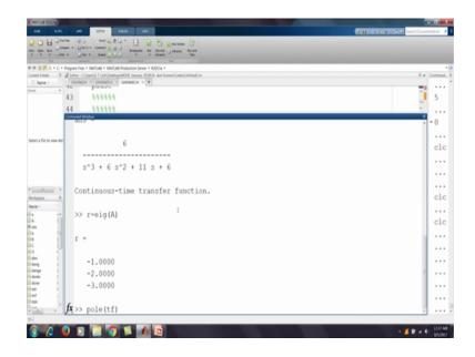
So, we get here the roots minus 1 minus 2 minus 3 and the same value we can because these are the poles of the system. Same value we should get also from the transfer function and so, if we give the command pole tf because this is a transfer function tf or sorry so, here we have pole tf num, den so, if we do pole tf num comma den.
