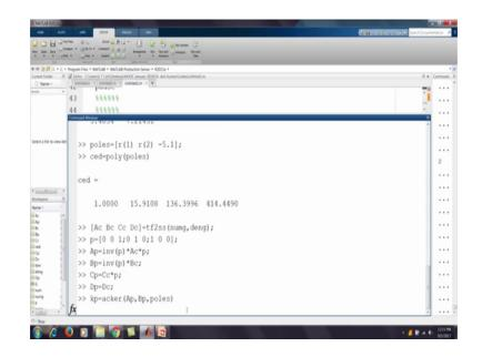
So, we put the third pole at 5.1 minus 5.1 so, we get poles that is poles equal to, here r1 so, r1 is this pole minus 5.4 plus 7.2 I then the second pole is r2 r 2 and then the third pole is minus 5.1 so, here minus 5.1. Now, we want the desired characteristic polynomials with these poles. So, ced equal to polly poles. So, this is the polynomial so, s power 4 plus this s cube plus this s square plus this value that is the polynomial and we can find the values of state space matrix.
