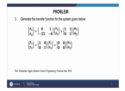
So, here generate the transfer function for the system given below. So, we have this state space model, but here we can see is the are the 2 inputs u1 and u2. Earlier we had here
