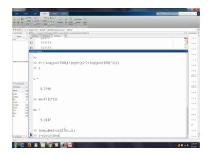
What damping we are getting about 0. 6. Now, omega n that is natural frequency we will get 4 by so, z into ts. So, we will get 4 by because natural frequency we can get by 4 by zeta into settling time. So, we get this natural frequency that is 9.0147.
