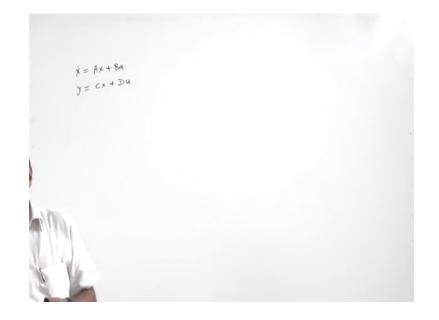
So, state equations we write like x dot equal to Ax plus Bu and y equal to Cx plus Du, here we know that different type of matrices A, B, C and D. We discussed in the lectures of week 7 about state space and how to transform from transfer function to state space, how to transform from state space to transfer function, then how to design a controller and how to determine the controllability of a system.
