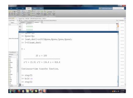
So, here I think we design the we design the state space feed by gains so that the system earlier system that is 20 s plus 100 by s cube plus 5 s square plus 4 s can give this percentage overshoot of 9.5 and settling time of 0.74. And so, here we first find the desired poles  $r_1$ ,  $r_2$  and we put the third pole at minus 5.1 so, that we can cancel the 0.
