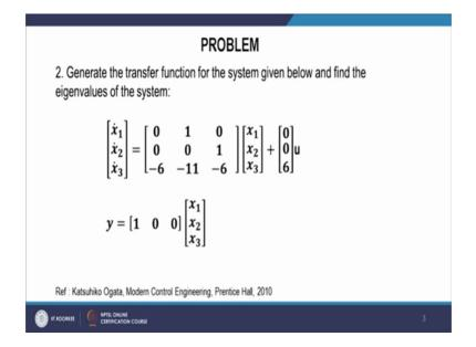
That is problem 2 so, here generate the transfer function for the system given below and find the Eigenvalues of the system. So, here we see this system is given in state space and we have to find the transfer function for the system. So, here A matrix, B matrix, C
