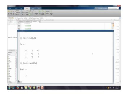
So, Rank we get 3 so, we know that the system matrix is of order 3A and Rank is also 3. So, this system has this is controllable because it is equal to the order of the system matrix.
