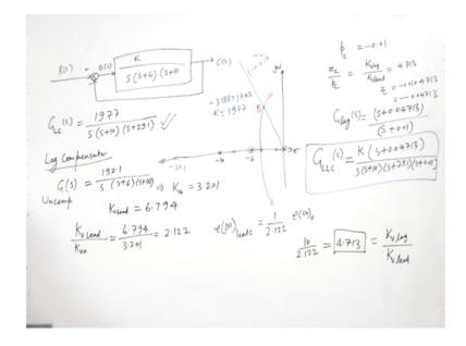
So, here we see that when we put the compensator 0 at this pole location they will cancel out. So, this 0 at S plus 6 concerned this pole system pole at S plus 6. So, this is the compensated lead compensated systems transfer function now we have to go for lag compensator. So, lag we have to design, so we know that the uncompensated system has. So, G S was and we had the gain K equal to 192.1 by S S plus 6 S plus 10 and from here we can find K v 0.
