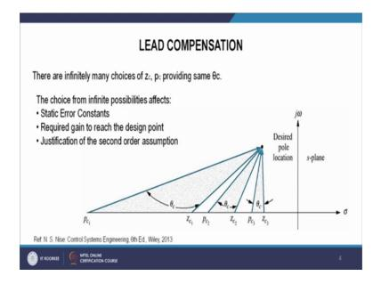
We can find this theta c such that there are several options to find to set this theta c, so that we can reach to the desired pole location. So, we can put like here z the pole the 0 and pole, so we will have this angle and we are going to have some desired pole location and this option also will give us the same desired pole location and similarly this option that is the third option.
