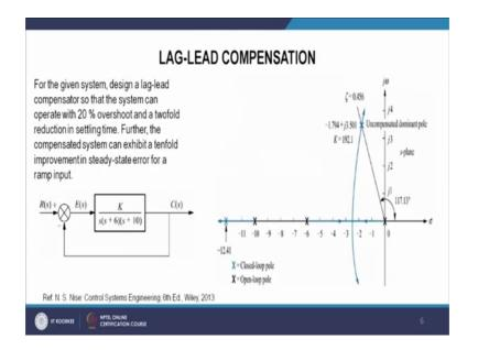
So, here we will take one example for this, so let us take one example and in this example we will use both lead and lag compensation to design for the transient response as well as the steady state error. So, here we have a question that we have this system and this system has this is our g s k g s and this is C s.
