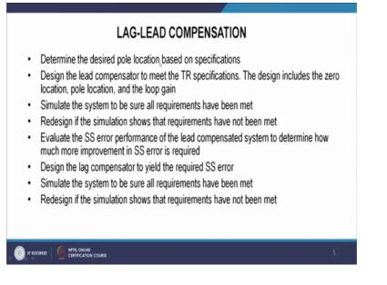
So, did the pole location is mainly decided by the transient response requirement like percentage overshoot settling time peak time and. So, we will find the desired pole location and for that pole location to obtain we design the lead compensator to meet that transient response specification, and when we use the lead compensator we will get that we add 0 and a pole for the compensator and some gain we will add to this in this design.
