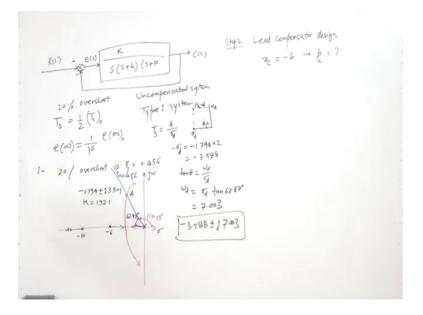
So, we have to design a lead lag compensator, so that for 20 percent over suit, we get the dominant poles at 20 percent overshoot and the settling time is half of the uncompensated system.
