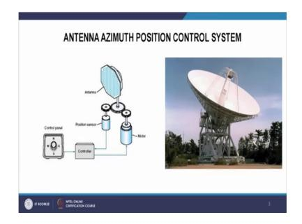
So, this is a radio telescope antenna, and this is your physical system. We have certain requirement of the performance specifications of this system. Suppose, this is a system we want to see the effect of a particular system parameter on the performance of the system.
