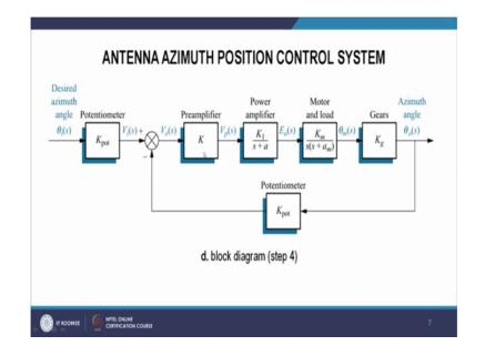
And so, there is transfer function each block has certain input, certain output. And that summing junction then input output. So, these each component can be represented as input output block diagrams.
