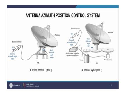
So, we have a physical system, now you see in this antenna, we are giving a input, that is desired azimuth angle input at the input of the potentiometer. So, there is a potentiometer shaft and and that shaft we are rotating. We are giving some angular input. And we want
