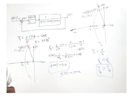
So, because this pole is at origin and we put at 0.1 close to this. So, that now the system type is increased, because this complete transfer function will have one pole at origin. So, the system type is increased and therefore, when we have 1 S here this 0 will keep K P infinite and K P infinite will keep this steady state to tend to 0. So, we will get this steady state now, what happens to root locus. So, we have this point. So, here is minus 1 minus 2 and here is minus 10.
