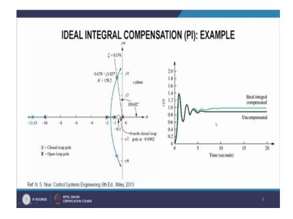
So, here we can in this diagram we can see the response of the 2 system. So, this is uncompensated system and we can see that uncompensated system is of course, there is this is the transient response characteristics, but the steady state error is large; however, with the ideal integral compensation we have increased the we have improved the steady state error because steady state error is tending to 0 and at the same time we see that settling time is larger.
