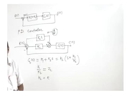
Now, this PD controller is proportional plus derivative. So, we have this RS here is proportional part let us say that is K 1 and then here is the derivative part and here is the G S and here is C S and derivative means we have K 2 into S. So, Laplace transform of a derivative. So, we have a derivative. So, d by d T function. So, the Laplace transform is K 2 S. So, in time domain it is derivative d by d t, but in s domain it is K 2 S.
