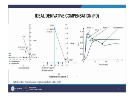
Now, we want to because if we want to have a PD controller we have to add here zero. So, here it should be K S plus z c this is the compensator PD compensator we are going to add 0. So, let us we try three conditions we add and check whether we are adding 0 at minus 2 minus 3 and minus 4. So, we are adding this z c is 2, 3 and 4. So, z CS plus 2. So, we are getting S equal to minus 2 here this zero. So, first condition is we are going to add a 0 at this location itself.
