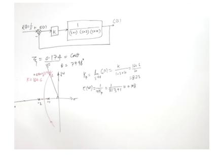
So, we can have let us take the example. So, we have this system here is the gain K. So, here we have we are giving the step input. So, we want that this is the system and we can see that here there is no any in this system there is no any pole at origin because there is no any S. So, this is type 0 system and this type 0 system is subjected to step input.
