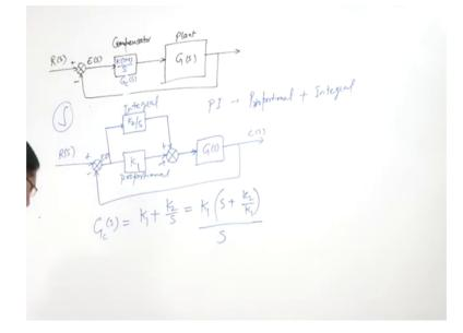
So, here we say that the PI controller, that is have 2 parts proportional plus integral and how with these 2 parts we can get the equivalent transfer function for these PI compensator.
