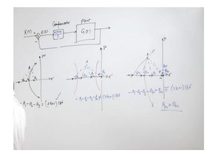
So, we have input we have this E s here K and G s. So, let us say this is gain and this is our plant. So, this is our plant and if we plot this root locus for this let us this G s has three open loop poles here and we have root locus and we have a point here A. So, here these angles theta 1, theta 2 theta 3 and we have these are all 3 poles. So, minus theta 1, minus theta 2, minus theta 3 should be equal to 2 K plus 1 180 degree.
