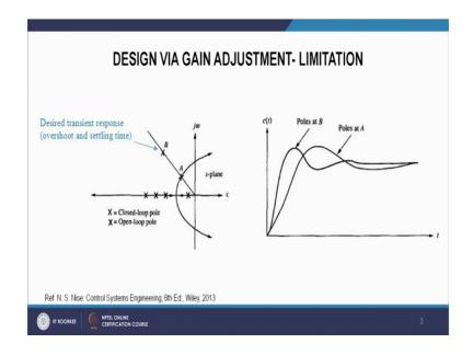
However, in this root locus we are forced to select a point only on the root locus because that root locus is a locus of closed loop poles when gain we varied again; however, what happens if we want to design the system for a point that is not on the root locus, so we can say that.
