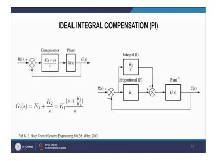
Now, how to deep resent this root locus, how to represent this ideal integral compensator compensation. So, we can see that here we have K s plus a by s. So, the we can represent it as individual circuits of gain and integration, so individual circuits or.
