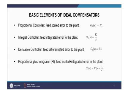
By scaling the error of the plant, so if we have here this is the our input this is our E s. So, here if we add some proportional compensator let us say k. So, K times E s will enter it to the input of the plant, so this is plant and here a gain is proportional controller.
