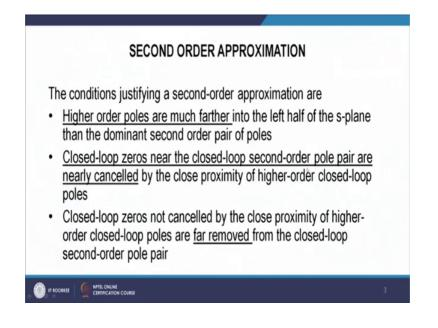
So, closed loops 0 near the closed loop second order pole pair or can be canceled by the close proximity of higher order closed loop poles. So, if we have 0 here, it will affect the response of this system and this role of this 0 can be only canceled if this third higher pole is linear to the 0.
