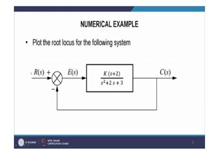
So, we have to plot the root locus for the following system. So, here is this input R S and there is error from E S. This is the K G s, that is K is the gain and this is G s and this is the output here unity feedback system. So, H s is 1.
