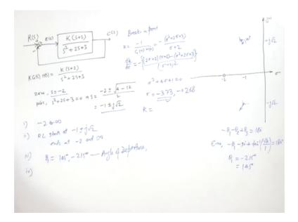
So, we have here this G s is K s plus 2, s square plus 2 s plus 3 and this is C S and unit feedback system here. So, we have to plot the root locus for this system. So, here let us, we have to plot here. So, here sigma this is j omega axis. So, the first thing is we have to locate. So here, K G S H S equal to K s plus 2, s square plus 2 s plus 3.
