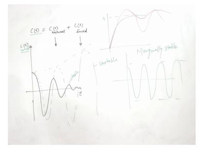
So, a the total response of a system is equal to, C t natural plus C t forced. So, here this natural response that is due to the, systems internal characteristic and this is due to the
