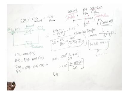
So, this is a transfer function and we can find the closed loop transfer function, because this is the forward loop forward transfer function, this is feedback, we have to find the equivalent transfer function of this system, and this we can find we can write C s equal to E s into G s, C s equal to E s into G s, and E s equal to R s. So, this is plus this is minus R s minus H s into C s.
