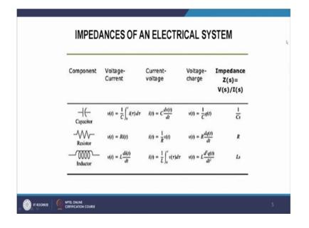
The capacitor has impedance 1 by c s, register has impedance R and inductor has impedance L s. So, we can convert the circuit to an equivalent impedance circuit. So, let us convert these. So, here is v s, this is R 1 R 2. This is L s, this is 1 by c s, and here is v c s. Here is I one s, and this is I 2 s.
