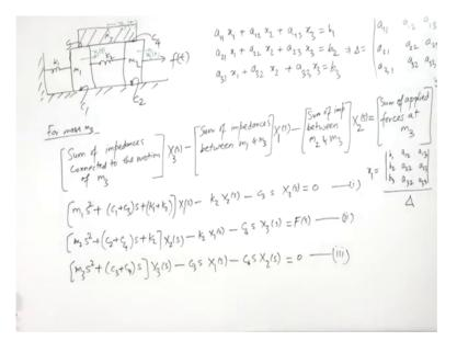
Minus sum of impedances between m 1 and m 3 into x 1 s. Minus sum of impedances between m 2 and m m 3 and x 2 s and some of applied forces at m 3. So, your sample sum of impedances connected to the motion of m 3. So, they are the m 3 s square plus c 3 plus c 4 s x 3 minus some of impedance between x 1 and between m 1 and m 3. So, between mm m 3 c 3. So, c 3 s into x 1 s minus here between m 2 and m 3 c 4 s into x 2 s. And that is equal to there is no any force applied here.
