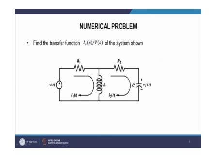
Resistance R 1 R 2 inductor L and capture c. And there are each current I 1 t in this loop first loop. And I 2 2 t in the second loop and here is the output voltage we are reading at the capacitor that is v c t.
