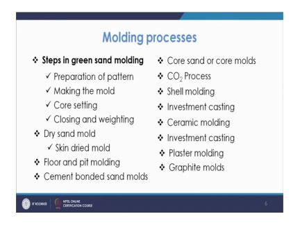
If you talk about the greensand molding in that these are the steps that is once you prepare the pattern then make the sand is that we have seen in the earlier lectures earlier slides. So, you make the mold and then core setting is done. So, code will be placed and it has to be seen that it is at proper place and closing and wetting of the cores is also seen that core should be towards the drag half otherwise it will floats. So, if it has to be in the drag of portions.
