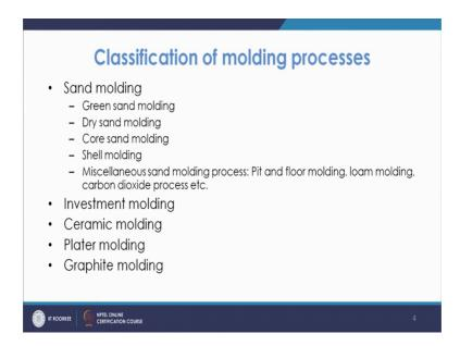
So, as you discussed we have the sand molding there we discussed about the green strength. So, similarly green means you have the moisture. So, based on that when you are doing the molding process with the green sand which has a moisture in it and the moisture gets evaporated, it gets the strength slowly because the moisture will be evaporated once the liquid metal is poured into the cavity.
