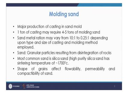
That depends upon the type and size of the casting and different type of molding methods.
