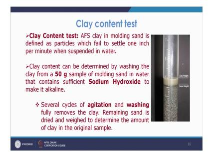
So, clay is basically defined as that particular you know particle which basically settles which is not which is failing to settle at certain rate.
