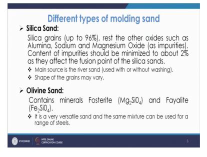
So, basically it is versatile sand and the same mixer can be used for a range of steel. So, that it has the special quality.
