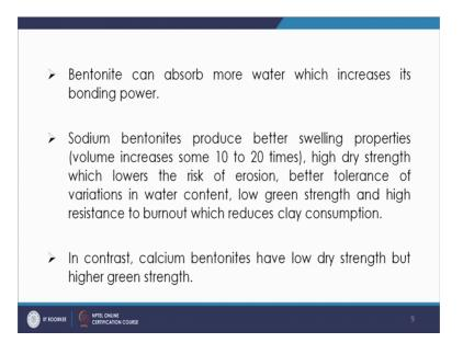
So, bentonite has the property that they can absorb more water, increase the binding power it has the, it is it will be producing the swelling properties. So, volume will increase and then it gives sodium bentonite gives the high dry strength which lowers the risks of erosion better tolerance of variations in water content like that. So, you have the low green strength or so. So, these and in contrast you contrast you have calcium bentonite which have opposite properties. So, like that.
