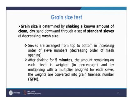
So, as we discuss that the grain which you collect you are getting you know collected from the riverbeds or from any other source they are of different sizes and shapes. Now, the size basically grain size affects the properties of the molding sand like its refractoriness permeability strength or so. So, we need to have standard where we can say that yes this is the size which is suited for that purpose.
