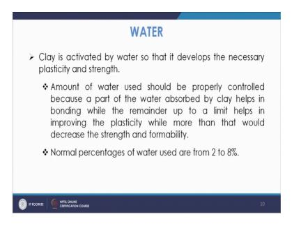
Water is basically, clay will be activated by water. So, that the binding is between clay and clay using water. So, what happens? The clay will surround the sand particles and they will be binding between water I mean clay and clay particles. So, basically that is activate clay is activated by water and you need one temper water that is required for binding, more water will provide more plasticity and that basically increases the permeability or flowability are decrease the strength.
