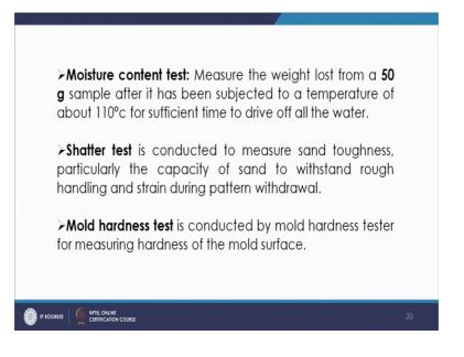
So, you are heating it for certain time moisture will be gone at 110 degree (Refer Time: 33:00) for sufficient time and the difference in the weight will talk about the moisture content test.
