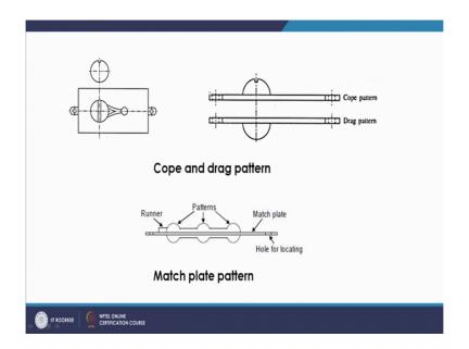
So, this will be there as a pattern plate on that you have this is the projection. So, for the casting suppose, and this basically will be taken out. And then once again you have the another pattern plate, which you are using for the drag part, and then you are joining these two you are combining these two and you are getting such kind of the cavity, and the cavity you can further pour the liquid metal.
