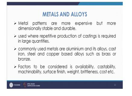
Commonly used metals are Aluminum and its alloys Cast iron steel and Copper based alloys such as Brass or Bronze which you can cast easily you have the material with good strength a good surface finish. So, that way these are the normal materials which are used you have the factors which you must consider is the availability cast ability, machine ability, surface finish weight brittleness cost.
