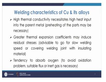
So, now the again the challenge with copper is that since its thermal conductivity is quite high. So, you need very high heat input into the parent metal and for that even the preheating is required because the thermal conductivity being very very high, the rate of heat transfer also the rate of heat being extracted will be quite fast.
