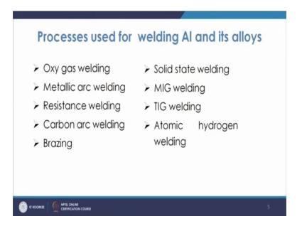
The process which are used for the welding aluminium and its alloys are like oxy gas welding then you have metallic arc welding, resistance welding, carbon arc welding, brazing solid state welding, MIG welding, TIG welding atomic hydrogen welding. So, these are normally the methods which are used for welding of the aluminium and its alloys, then the next material which we are going to discuss will be the copper and its alloys.
