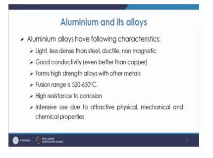
And very; so, then it is quite ductile and non magnetic then its conductivity is quite high even it is having better conductivity then the copper also, then a aluminium has the tendency to form the high strength alloys with other metals. Now, if you take the pure aluminium then pure aluminium is soft and it does not have much of the strength.
