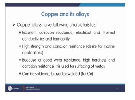
So, copper is again one of the very important non ferrous material which has extensive use and because of because it has very good properties. So, we will discuss first of all its property and then the challenges related to the welding behaviour of this material. So, copper alloys now they have very good corrosion resistance electrical and thermal conductivity and formability.
