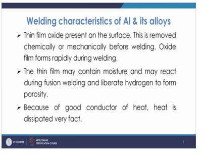
So, we are going to discuss something about the welding characteristics of aluminium and its alloys. Now, if you talk about the aluminium the important thing in the case of aluminium is that you have the thin oxide film which is present on the surface. As we know that in aluminium you have the oxide of aluminium 1 2 o 3 on the surface and this is removed chemically or mechanically before welding, you have to remove them and the this oxide film basically rapidly forms during the welding also.
