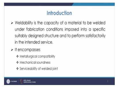
So, when we talk about weldability so, it is the capacity of a material to be welded under fabrication conditions imposed into a specific suitably design structure and to perform satisfactorily in the intended service. The thing is that you are welding the material or joining, sometimes a you have different conditions you may have the joining with one way like you may use the you know flame welding or you may use arc welding or you may use the non-conventional welding processes.
