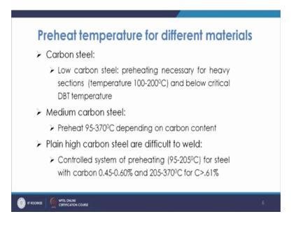
Because when the carbon content is smaller than you do not require that much of a preheating, but so a when you have a carbon content to lower side then you do not require the preheating because, the harden ability is less in that case harden ability increases with the carbon content.
