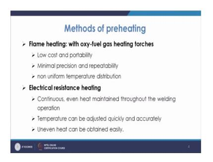
Now method of a preheating, so when we talk about the method of a preheating, how we can do preheating like you may do with the flame. So, you have you can use the oxy fuel gas heating torches, so you have a torches of diameter then you have you have from there you can if you are with the supply of the gas, you can generate a flame of a different type like maybe like you we know that we have they have 3 types of flames.
