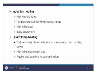
So, then you have the induction heating, a induction heating is further the another you know mechanism by which you can do the heating. So, it has the advantage of like you
