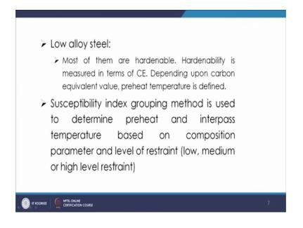
So, that is a PCM also or it will be effect it will be simply a function of the similar to that carbon equivalent and once we get that value then basically what we do is, we determine the preheat and inter pass temperature based on the level of restraint.
