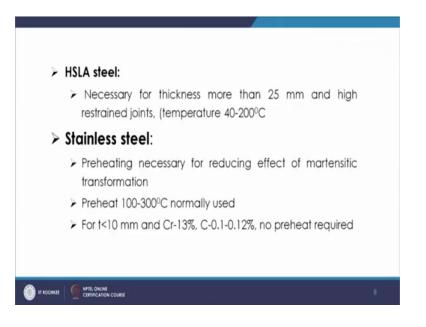
Now, we will go to the other kind of a steels like a for HSLA that is high strength low alloy steels, in those cases when you have the thickness of more than 25 mm and you have the high restraint joints then temperature is about 4 at 10 to 200 degree centigrade is taken.
