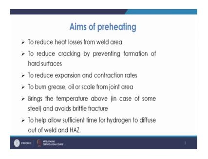
So, as we discussed that the aim of preheating is to reduce the heat loss from the weld area, to reduce the cracking by preventing the formation of hard surfaces or a hard phases many a times hard faces like martensite or so to reduce the expansion and contraction rate.
