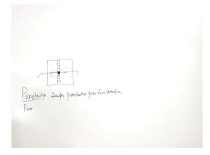
this is the welding. So, here once you are heating at this point now the heat has to extract from here and from here, now if the thermal conductivity is high it will quickly pass through it and then it will go to the surroundings.
