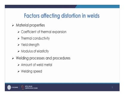
So, the materials which we are basically using for welding process they have it is own specific properties and as this properties vary from material to material. So, the expansion characteristics or the distortion characteristic will also be changing.
