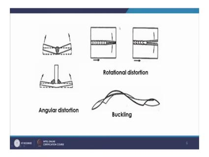
This is the example of rotational distortion, now this is observed at the at ahead of the point of the welding and when you are welding the seats then you many a times you see that these seats when you are doing the butt welding of the seats then they come either closer to each other or they are basically in the distance between them is widened. So, in this case what you see is these 2 edges either they are coming closer or in this case they are going away.
