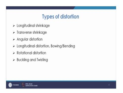
What are the types of distortion, how the distortion looks like ok. So, distortion is normally of these types like you have longitudinal shrinkage, you have transverse shrinkage, you have angular distortion, you have longitudinal distortion, you have rotational distortion and buckling and twisting.
