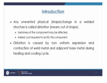
Structure is called distortions means anything which is going out of shape which is not in the shape which for which it is meant to be then it is said to be distorted. So, you know usefulness of the component may be affected.
