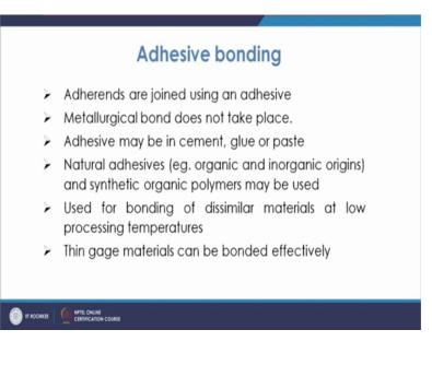
Then you may have the natural adhesive like organic and inorganic origins or synthetic type of organic polymers which are used. this is normally used for bonding of the similar materials at low processing temperatures and there is thin gauge materials which can also be bonded effectively.
