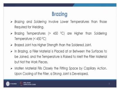
Now, the differ only by the property of the filler metal which is used like in the case of brazing it is braze alloy. So, for that similarly in the case of soldiering it is solder alloy. So, depending upon the strength or depending upon the melting temperature of these alloys you have either category as brazing or soldiering.
