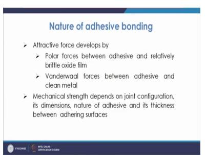
So, dipole creation that is between adhesive and relatively brittle oxide film, another is the because of the Vanderwaal forces which are generated between the adhesive and the clean metal. So, that is the concept of the strength which develops in the case of these adhesive bonding.
