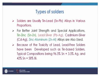
Solder in most of the cases because of it is quite low melting point and that too. If you look at the phase diagram of tin and lead you will have this eutectic which is which has even the quite a lower of lower value of melting temperature. So, that way it is quite popular for using as the solder material because with very small temperature increase it can be melted.
