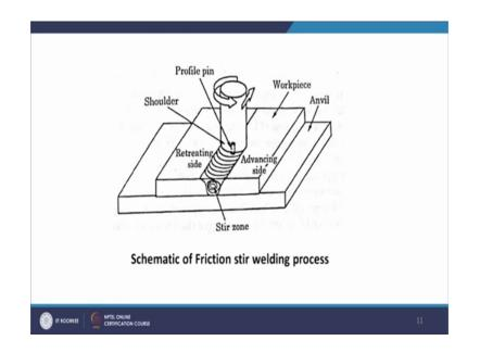
Now, this is the schematic of a friction stir welding as you know. in this case you will have a tool here this is in terms of a pin and then you will have this is as the profile surface. So, this is the shoulder cone known as and this pin basically goes into this recess and then it rotates and rotates and progresses along this the along this length.
