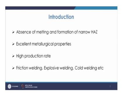
So, what happens in the case of solid state welding processes now, the thing is that in this case in the case of solid state welding processes you have absence of melting and formation of narrow heat affected zone. So, solid state welding means the parent materials which are the ones like mostly the bars or tubes.
