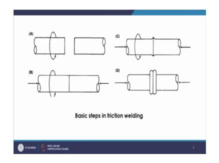
Now we will discuss about the sequence of the different steps which occur in the friction welding. So, as we see that you have steps A, B, C and D. Now, what happens that initially this is you see that there is rotation of A. So, A is rotated and B is stationary A is rotated and so this part is rotated another part is stationary. So, slowly, that will be brought together.
