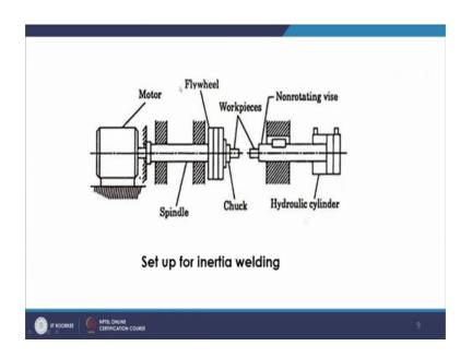
So, as you see that you have a flywheel attached here and then this is a spindle and then you will have nonrotating vise. So, that will be brought in contact with this and then that way since this is inertia of the flywheel is used that is why you we use this term known as inertia welding.
