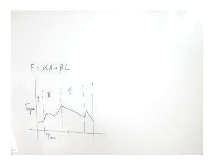
And, then after that this will be the third stage which; will where the plastic deformation takes place and then in the fourth stage again it will increase in and then it will be decreasing. So, that will be the final stage and in that final stage you are breaking and forging taking place. So, this way there are four stages in the case of friction welding taking place.
