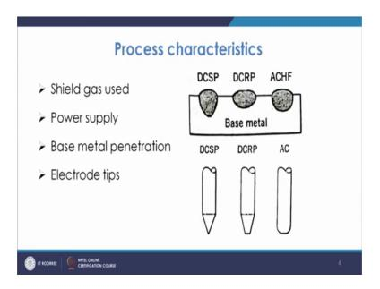
So, as we know that when we talk about the process characteristics the shielding gas used as we know that there are basically two types of shielding gases used helium and the carbon dioxide gas this argon gas and in the power supply and also because the carbon dioxide is also off let has been used in many applications because carbon dioxide is quite cheaper as compared to helium or argon.
