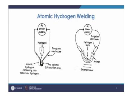
Now, in the case of atomic hydrogen welding what happens that here you have the mechanism in different way. Now, in this case what happens that the electrode will be same way produced between the two tungsten electrodes, but then the hydrogen gas is passed in between them? Now, what happens that the hydrogen molecule which passes as it comes in contact with this arc which is at higher temperature now that basically disassociates so, that breaks that hydrogen molecule into hydrogen atoms.
