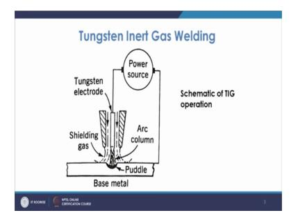
Now, coming to the variety of the gas arc welding process the most popular of these processes the tungsten inert gas welding it is also known as TIG process. So, either we call it as GTAW gas tungsten arc welding or tungsten inert gas welding process. Now, what we see is that in this schematic of this process you have the tungsten electrode which is used to only create the arc. So, the tungsten electrode we can use the DC or AC power supply.
